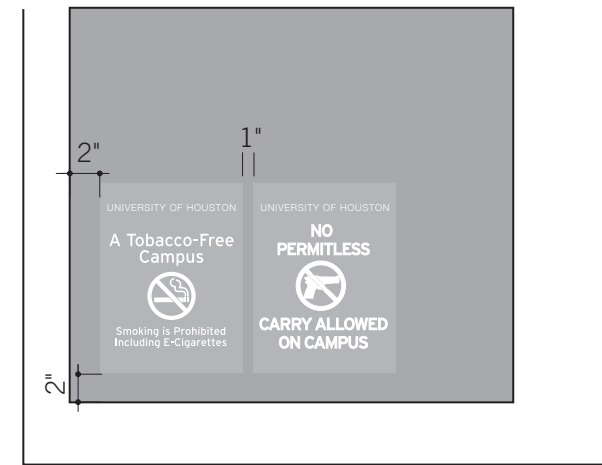
REFERENCE IMAGE TYPICAL PLACEMENT, MYLAR ADHESIVES
