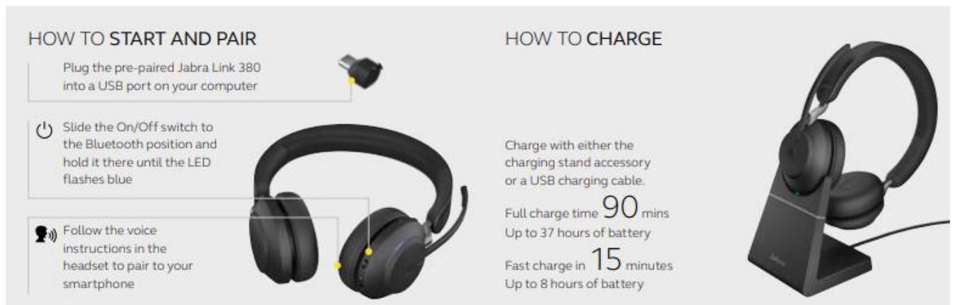
Charge with either the charging stand accessory or a USB charging cable.
